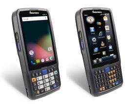
With its multi-touch, outdoor-readable screen, long battery life and highly accurate barcode scanning capabilities, the CN51 Mobile Computer offers unparalleled versatility and performance for mobile workers.
